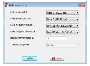
To configure LoRa<sup>TM</sup> parameters we must click *Modify* button with wireless network icon.
