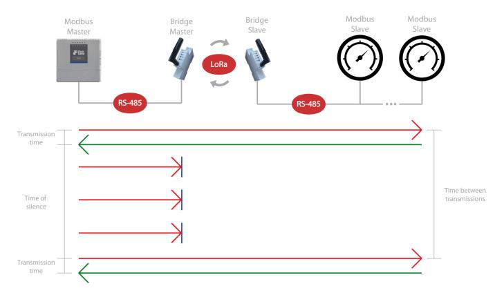
Based on these times, we establish 2 communication rules that must be applied at the Modbus Master. The first one is completely mandatory in order to establish communication with the Modbus slaves through a Bridge LR network:
